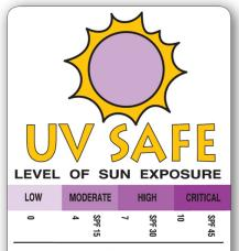
Expose the UV Safe Meter to direct sunlight for 20 SECONDS, then compare the color in the sun's center with the meter bar to find the approximate UV intensity.
